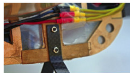
Strengthened with 1 mm ply, the U/C mounting caused no more problems
