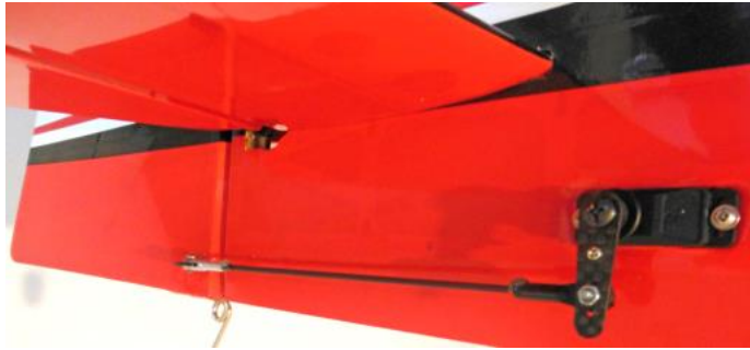
Rudder linkage geometry
