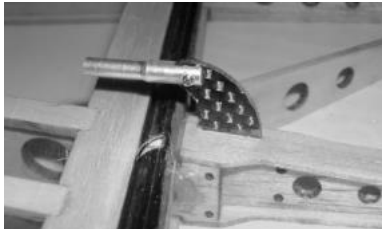
Test fit control horn
