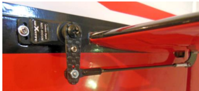
Elevator linkage geometry
