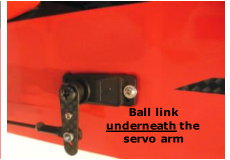
CF CNC machined rudder servo arm
