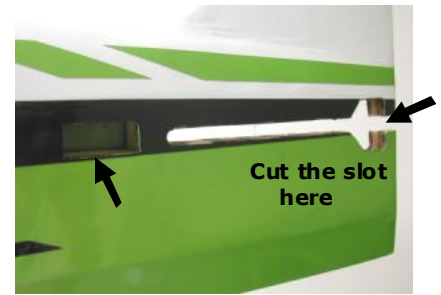
Stabilizer slot and Elevator Servo Opening
