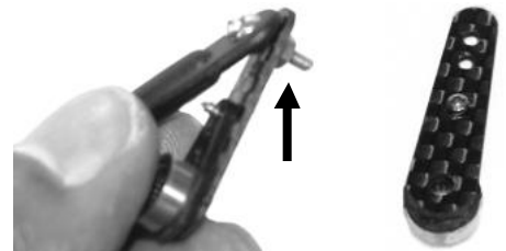
Secure the bolt with Loctite
