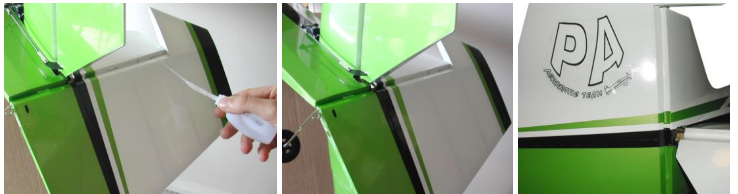
Deflect rudder to maximum before gluing the hinges
