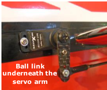
CF CNC machined elevator servo arm
