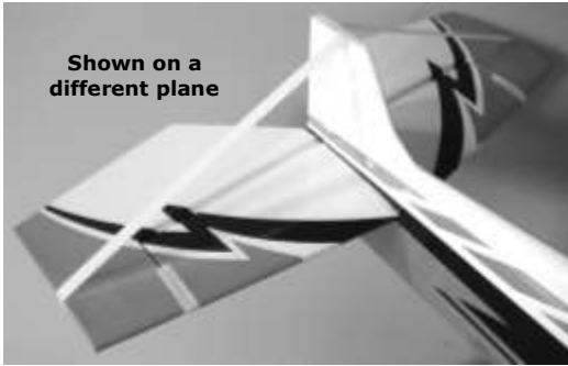
Apply epoxy to the stab center
