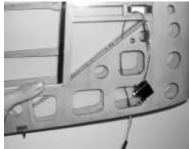
Feed the extension lead through
