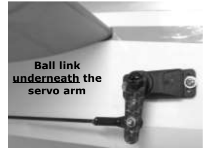
CF CNC machined rudder servo arm
