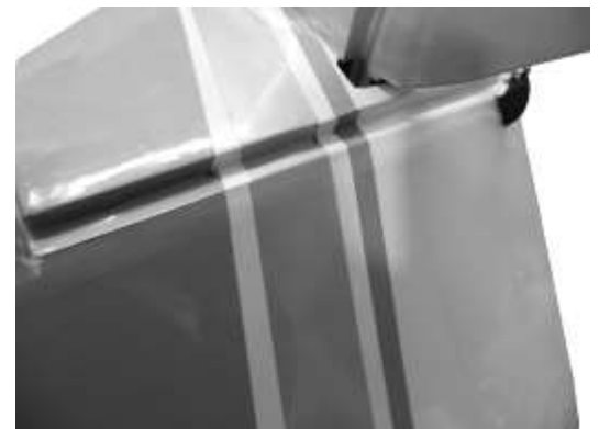
Seal the entire hinge gap while rudder is fully deflected
