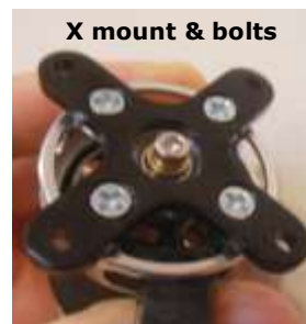
NOTE: Install the motor with the cables positioned downwards
