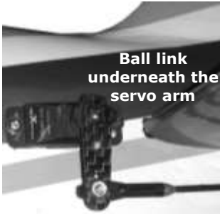
CF CNC machined elevator servo arm
