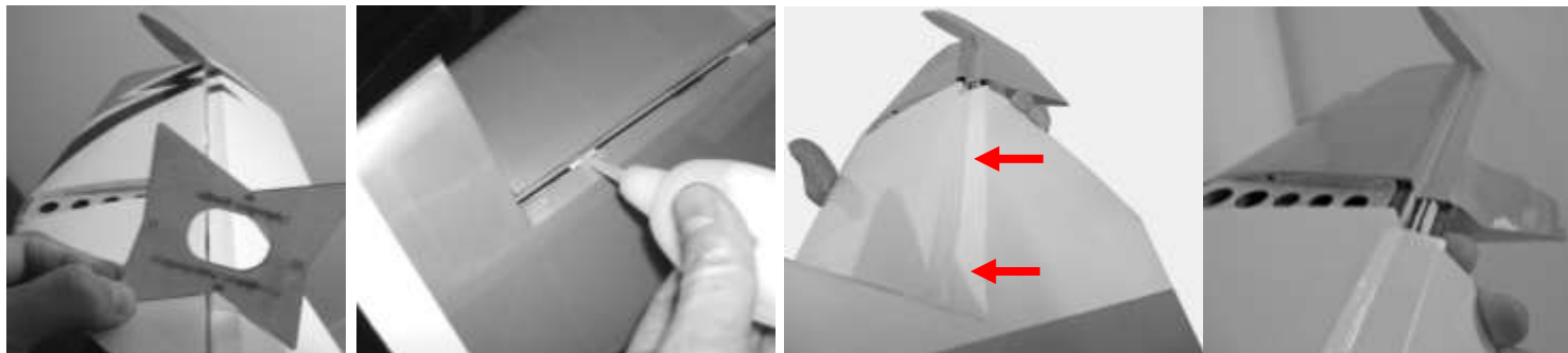
Deflect the elevator to approx 55° to set the hinge gap
