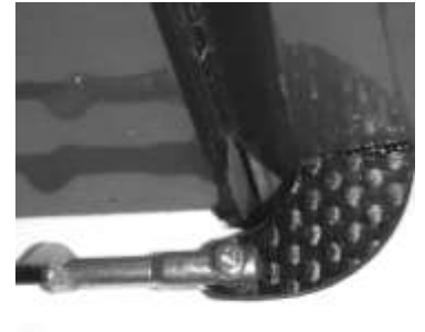
CF elevator control horn and clevis
