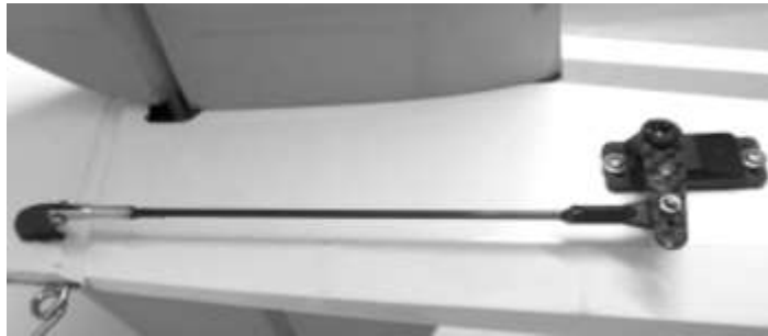
Rudder linkage geometry
