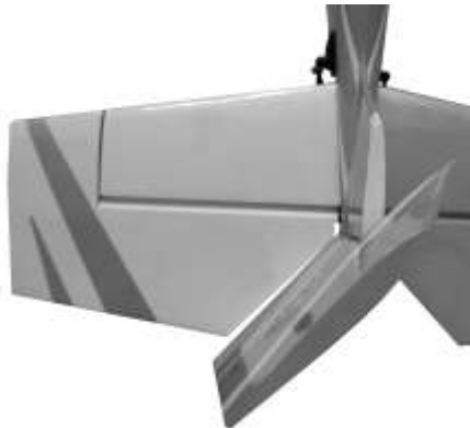
Deflect rudder to maximum before gluing the hinges
