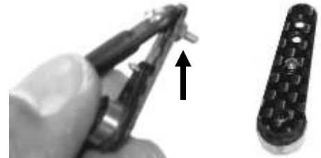
Secure the bolt with Loctite
