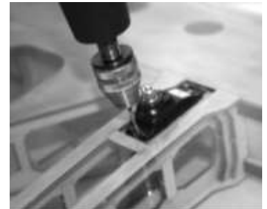
Drill the mounting holes with care
