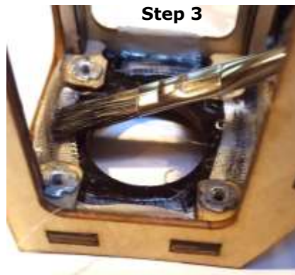
Step 3 Tuck in fibreglass cloth into seams
