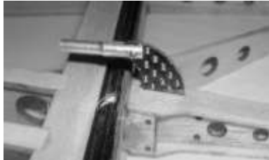
Test fit control horn
