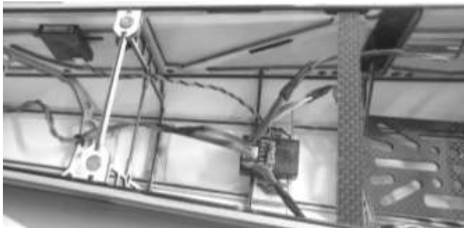
Spektrum 2.4GHz receiver installation
