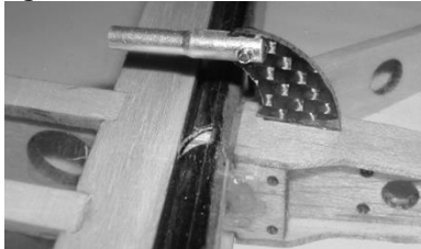
Test fit control horn
