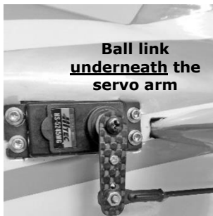
CF CNC machined elevator servo arm
