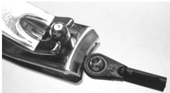
Trim the tab off the ball link
