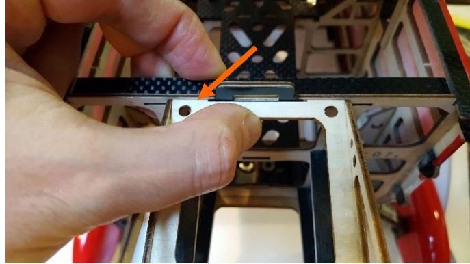
Hold the motorbox firmly with your fingers and apply a drop of CA (top and bottom) before applying epoxy
