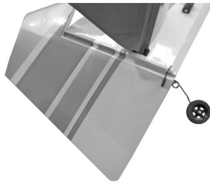
Place creased covering strips in the hinge gap
