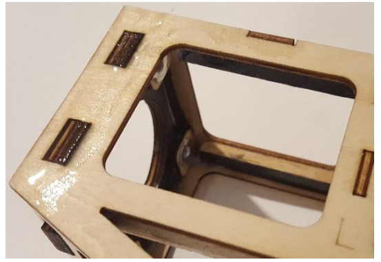
Apply epoxy over the motorbox front perimeter (including top and bottom sides)
