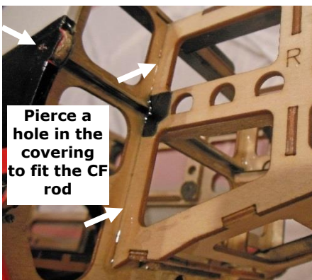
Epoxy ALL seams of the motor box with the bulkhead
