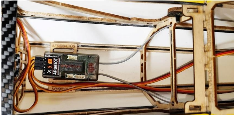
Spektrum 2.4GHz receiver installation
