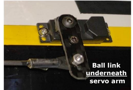
CF CNC machined rudder servo arm
