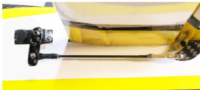
Elevator linkage geometry
