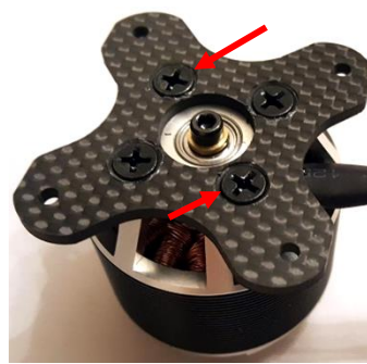
Bolts head must NOT protrude
