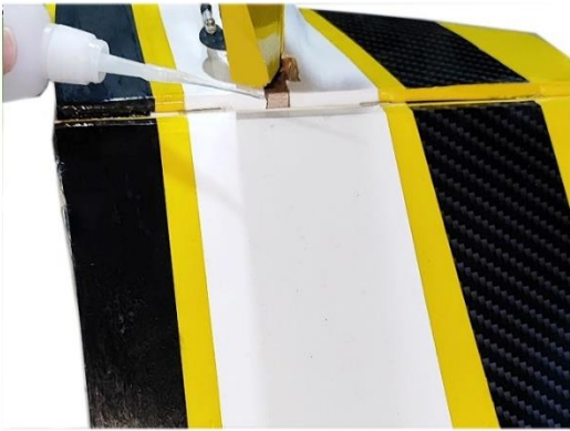
Deflect rudder to maximum before gluing the hinges
