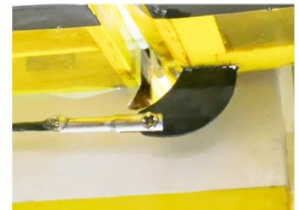
CF elevator control horn and clevis
