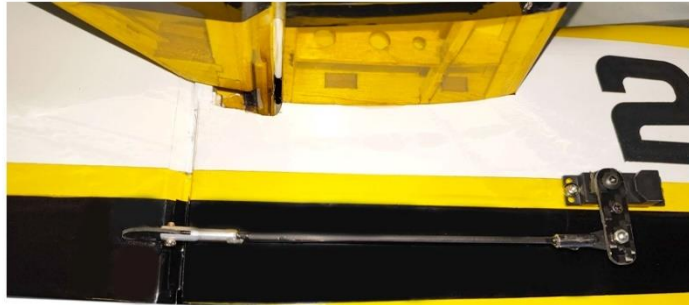
Rudder linkage geometry
