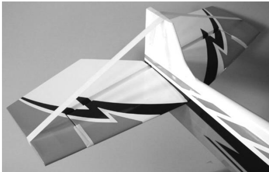
Apply epoxy to the stab center
