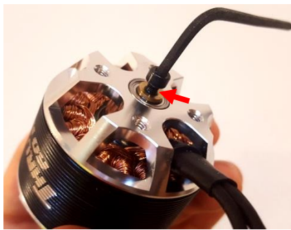
Apply Loctite to the retaining bolt
