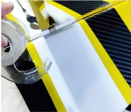
Place creased tape strips in the hinge gap
