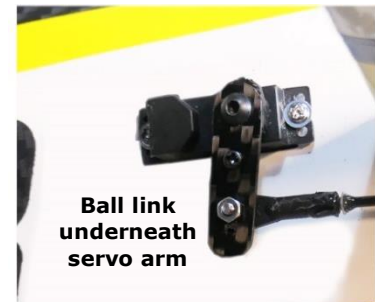
CF CNC machined elevator servo arm
