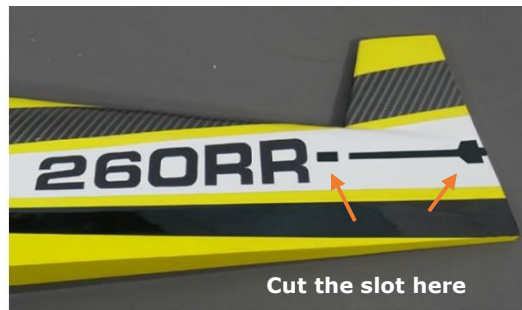
Stabilizer slot and Elevator Servo Opening
