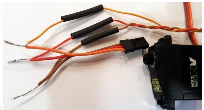
Solder and insulate each cable
