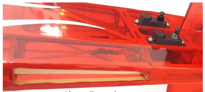
Air cooling exit
