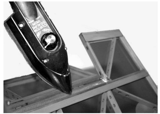
Iron in the covering strip
