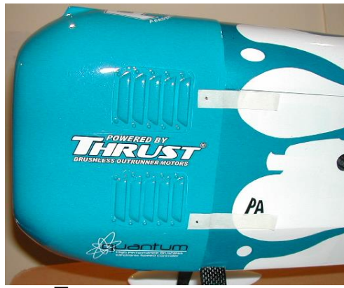
5 Fit cowling and drill
