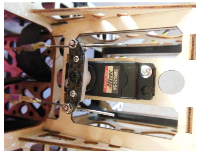
Install rudder servo in the motorbox
