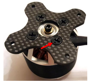
Counter sink motor bolts
