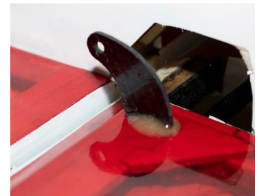
Elevator control horn
