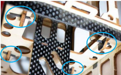
Glue motor box lugs and CF pins
