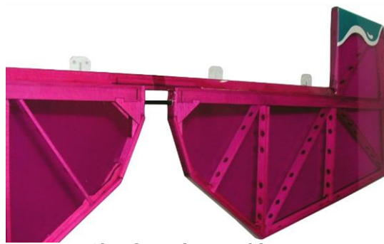
Glue four elevator hinges
