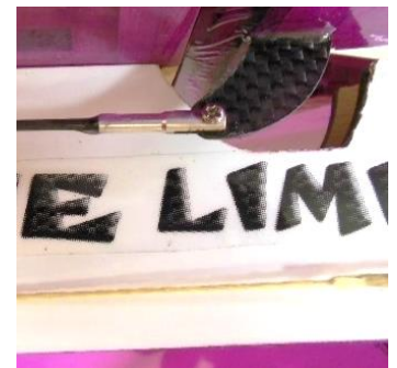
Elevator control horn
