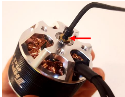
Apply Loctite to the retaining bolt
