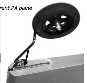
Apply Epoxy over the LG
