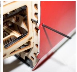
Pierce a hole in the covering to fit the rod
