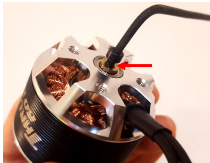
Apply Loctite to the retaining bolt
