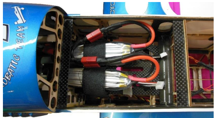
Batteries placed on their side and into the cowl
