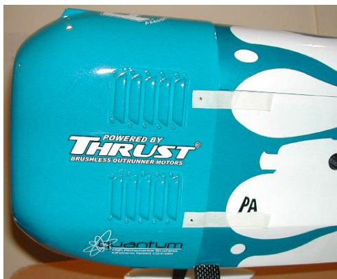
5 Fit cowling and drill
