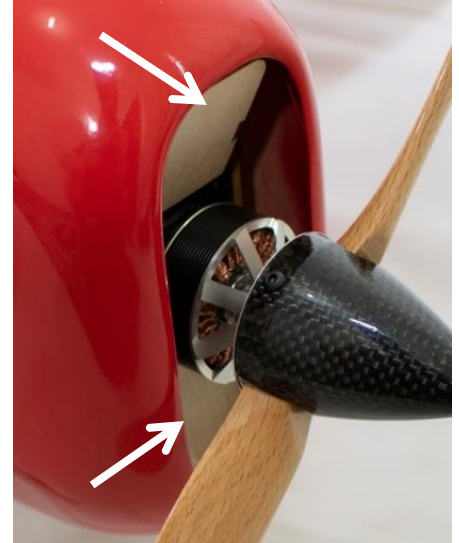
Install air baffles
