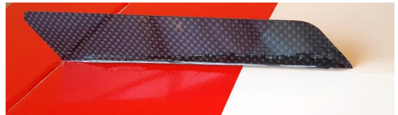
Apply a thin bead of epoxy along the entire seam
