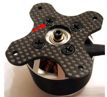
Bolts head must NOT protrude
