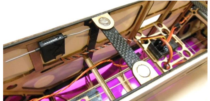
Batteries can be mounted flat or upright
