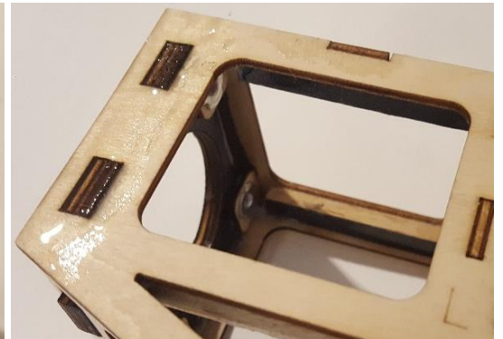
Apply epoxy over the motorbox front perimeter (including top and bottom sides)
