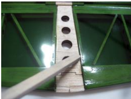
Apply epoxy to stab center
