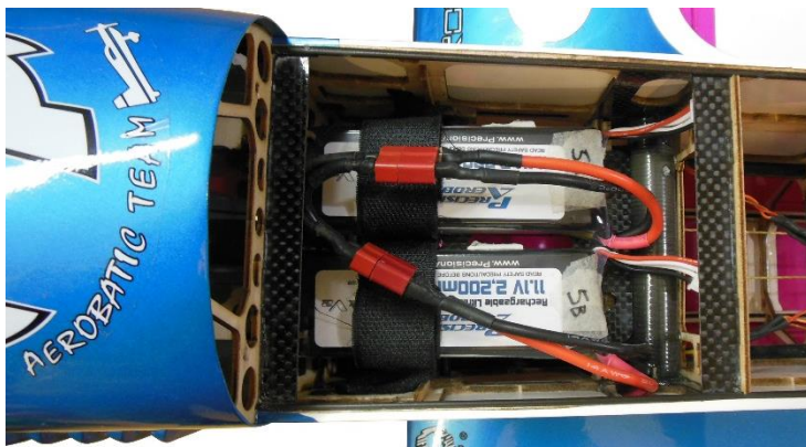
Batteries placed flat on the tray
