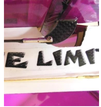
Elevator control horn
