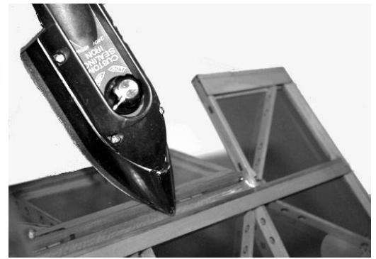
Iron in the covering strip
