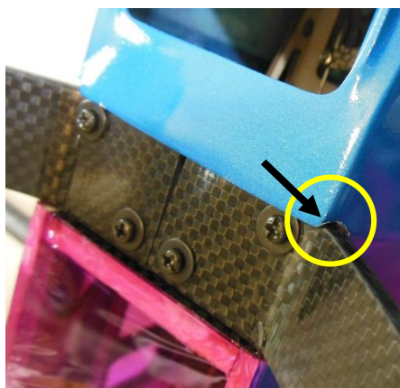
1 Notch the cowling to clear the LG
