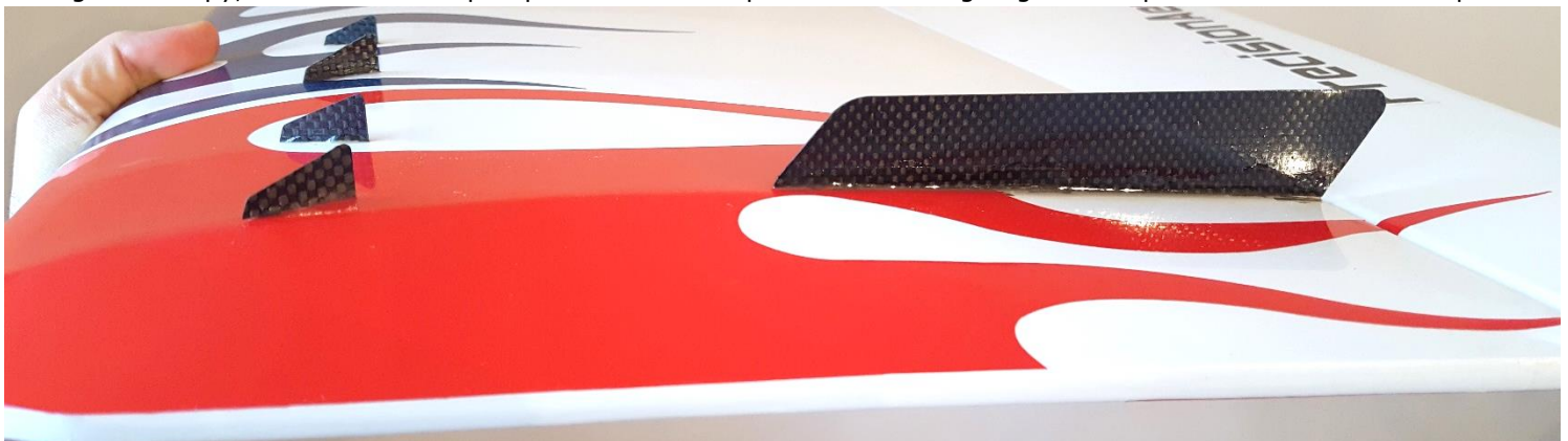
Apply a thin bead of epoxy along the entire seam
