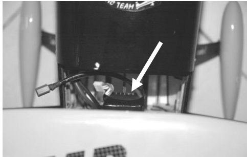
Battery aligned with the front CF tray
