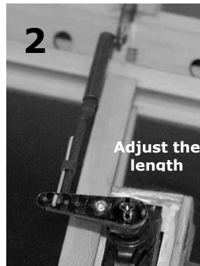
Servo arm at 90 Deg to the servo case
