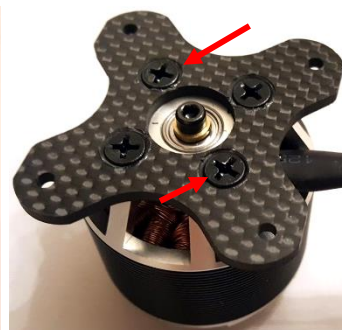
Bolts head must NOT protrude
