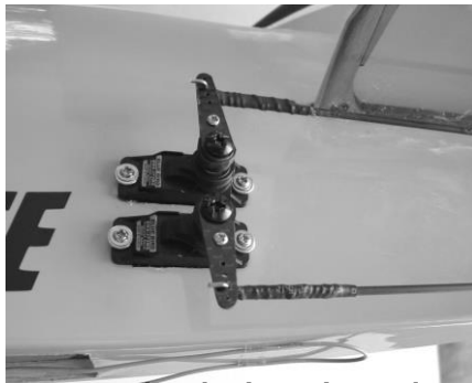
Note z-bend orientation and position on servo arm
