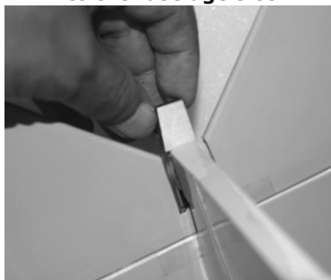
Insert balsa block into the fuselage slot
