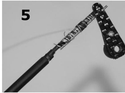
5 Soak string with CA and slide heat shrink tube in place
