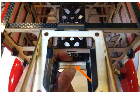
Hold the motorbox firmly with your fingers and apply a drop of CA (top and bottom) before applying epoxy
