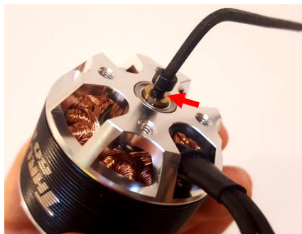
Apply Loctite to the retaining bolt
