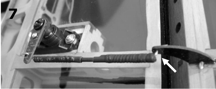
7 Note the Z-bends orientation
