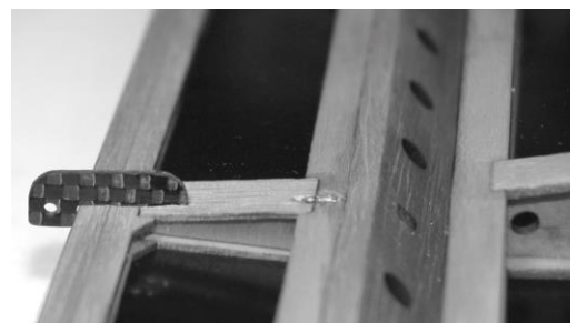
Keep a bit of the epoxy excess
