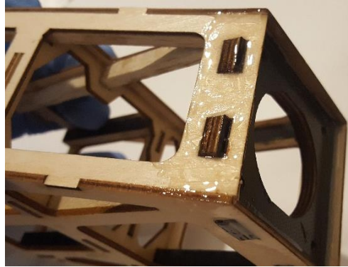
Apply epoxy over the motorbox front perimeter (including top and bottom sides)
