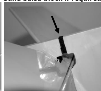
Sand balsa block if required
