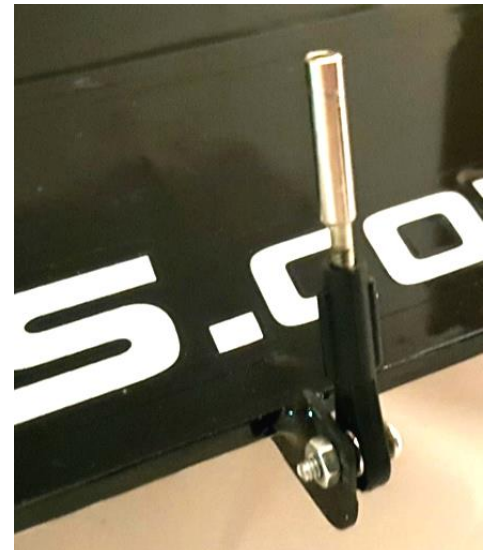
Ganging CF control horn (Bottom wing)
