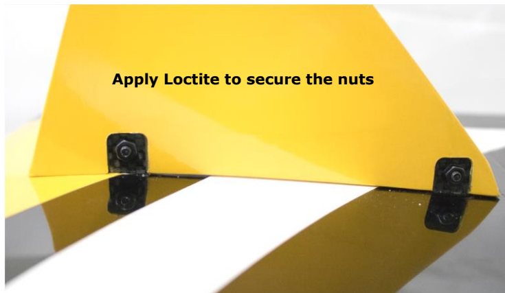
Minimize any gap with the wing
