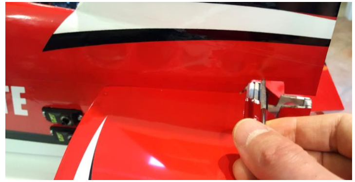
File a notch for the tube
