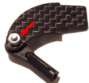
Secure the bolt with Loctite
