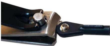
Trim the tab off the ball link
