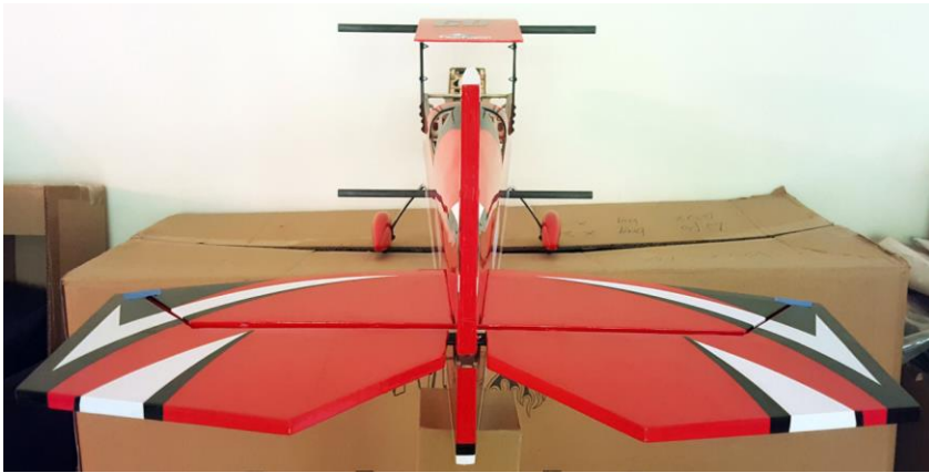
Fully deflect the elevator UP
