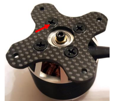
Bolts head must NOT protrude
