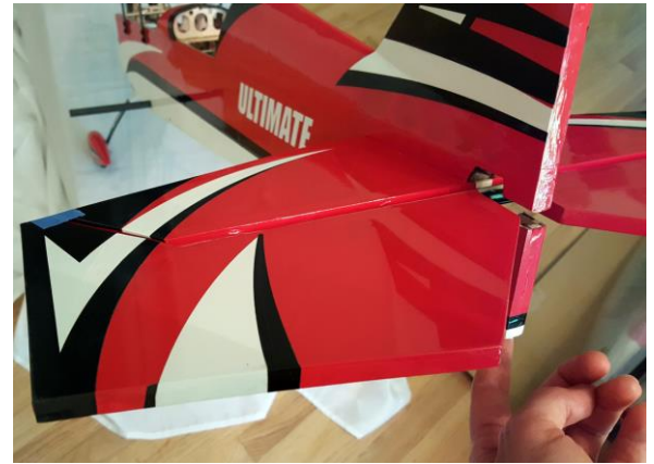
File a notch for the tube
