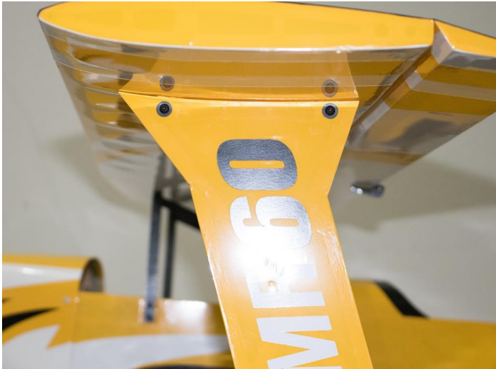
Minimize any gap with the wing
