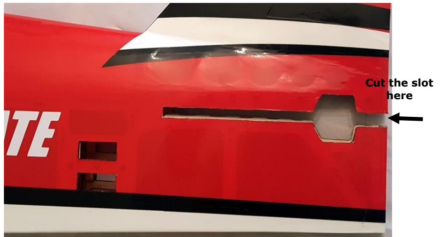
Cut the stabilizer slot
