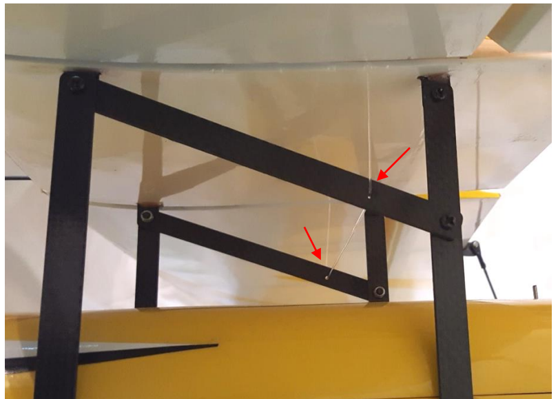
Fishing line through the diagonal cabane strut
