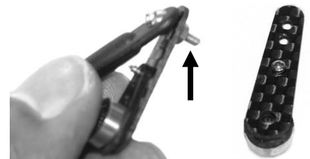
Secure the bolt with Loctite
