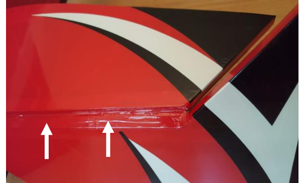
Place creased covering strip in the hinge gap and iron
