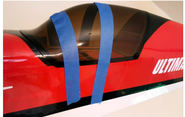
Hold canopy down with masking tape
