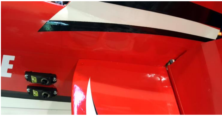
Fully deflect the elevator UP
