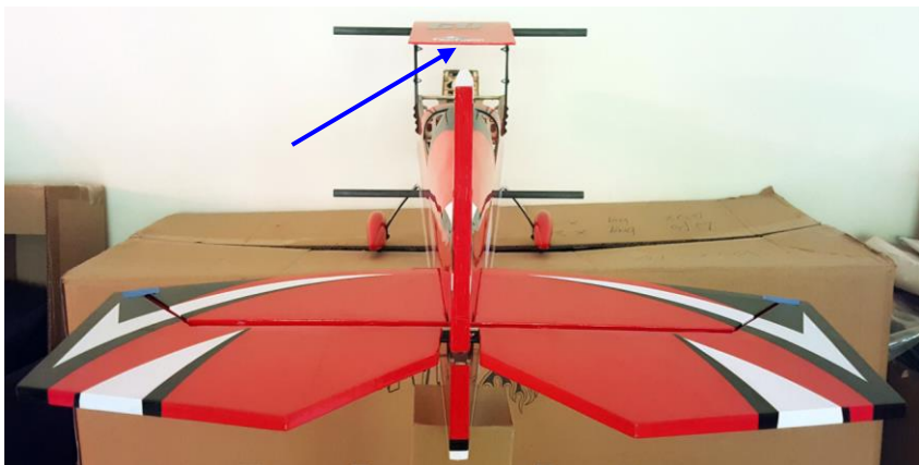
Inspect the cabane's Trailing Edge
