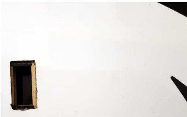
Aileron servo opening
