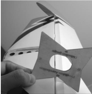
Deflect the elevator to approx 60° to set the hinge gap
