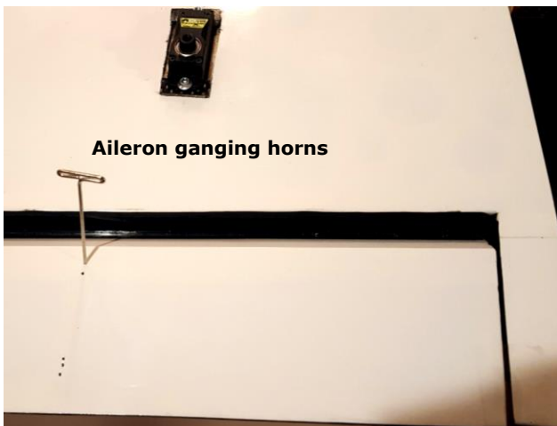
Make a few pin holes to expose the pre-cut slots
