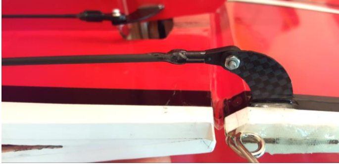
CF rudder control horn - ball link on top
