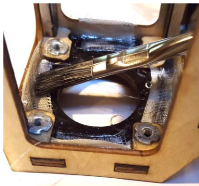
Tuck in fibreglass cloth into seams
