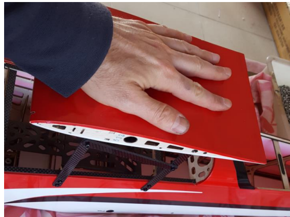
Press down while fastening the bolts
