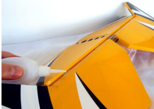
Gluing the elevator hinges
