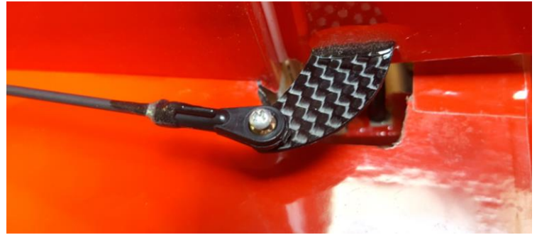
CF elevator control horn and ball link
