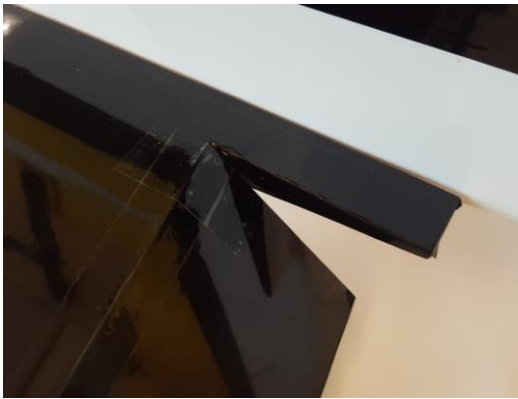
Piece of clear tape over the aileron root
