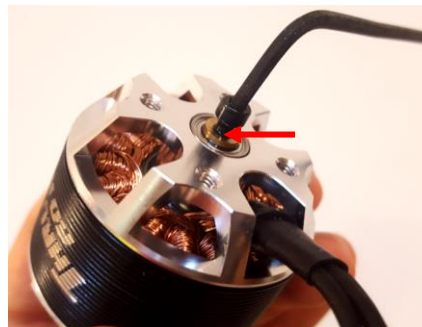
Apply Loctite to the retaining bolt
